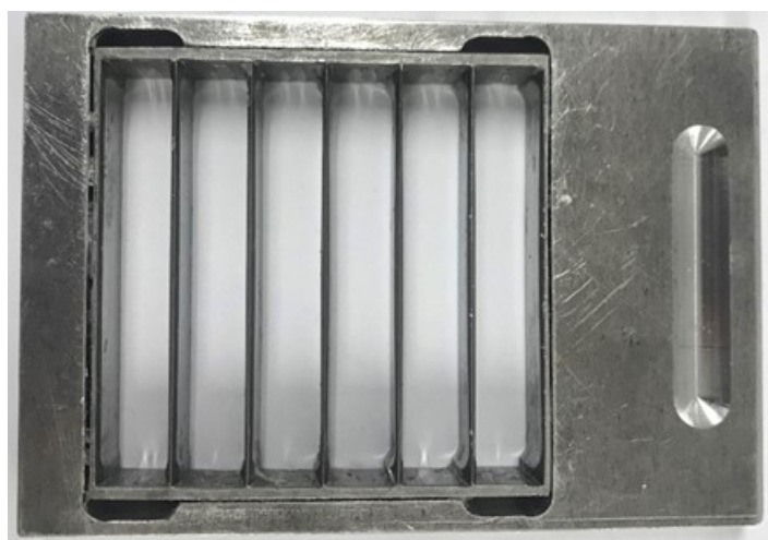
Figure 8: Ad-hoc 5-blade grid used for texture-extrusion analysis of boiled cassava roots
