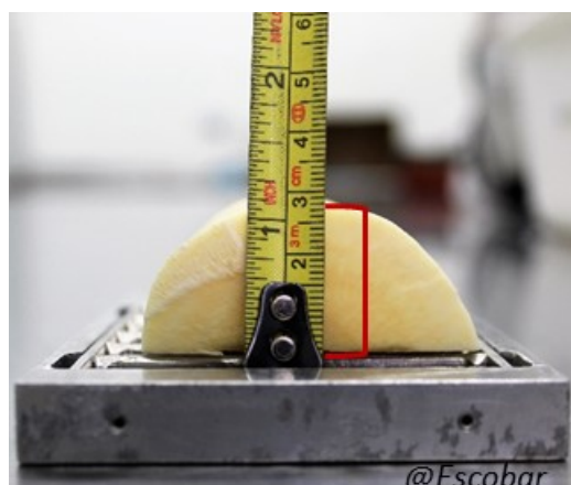
Figure 3: Minimum radius 2.5 cm for texture test
