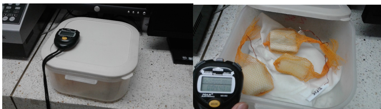
Figure 5: Cooling down of boiled cassava pieces for 10 minutes in a closed container to minimize moisture loss before texture analysis
