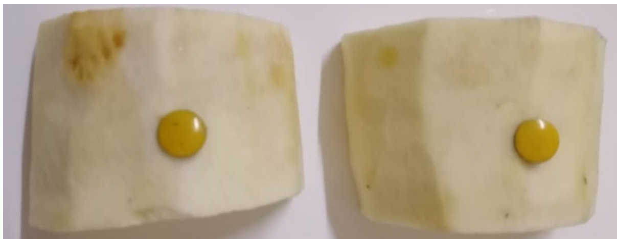
Photo 3: Half cylinder of boiled yam for penetrometry test
