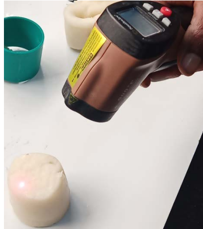
Figure 5: Monitoring of sample temperature using infra-red thermometer
