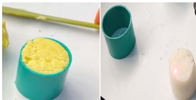
Figure 4: Cylindrical cup (4.0 cm long x 4.7 cm diameter) for sample preparation
