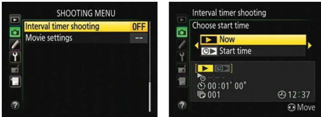
Figure 1 : Example of intervalometer settings.
