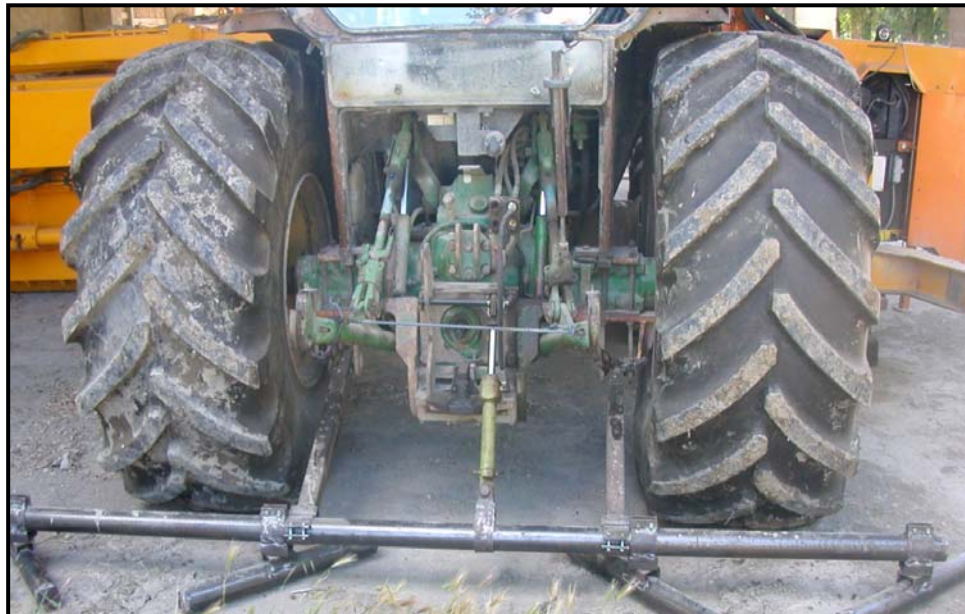
Efface traces rudimentaire a relevage hydraulique
