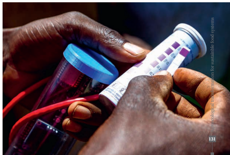
▼ Explaining the use of the Chameleon to determine soil moisture at three different depths.
