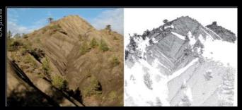
▲ Left: panoramic photograph; Right: 3D point cloud obtained by terrestrial lidar.
