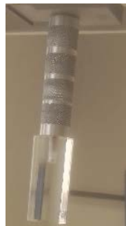
Figure 2. P/20P standard cylinder probe of 20mm diameter, Perspex (Stable microsystems).
