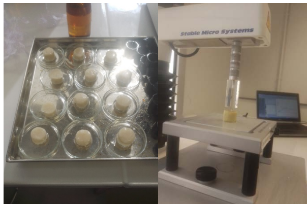
Figure 7. Moulded samples lubricated with paraffin oil before and during measurement.
