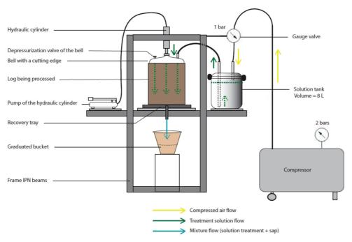
**Figure 1.** Scheme of the laboratory prototype used for the axial impregnation tests.
