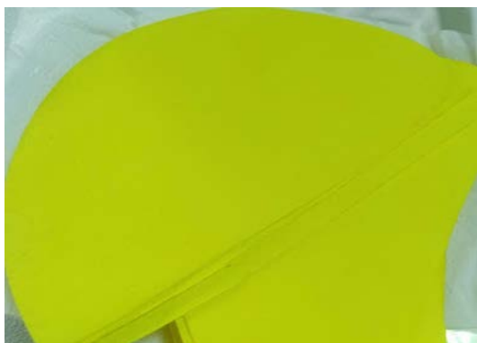
Figure 1: Freshly prepared picrate paper for qualitative determination of fresh root HCN content
