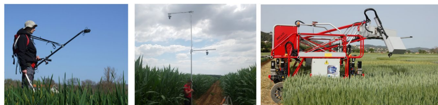
Fig. 3 Three acquisition systems used to build VegAnn. From left to right: handheld camera on the LITERAL device, camera equipped with a fish-eye lens and mounted on a probe, and cameras mounted on the Phenomobile. The individuals consent to the publication of the images.
