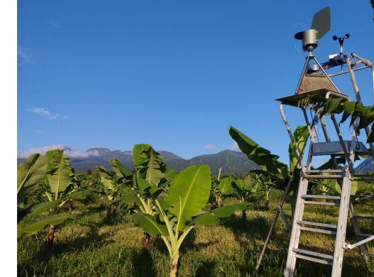
Burkard multi-vial cyclone sampler
