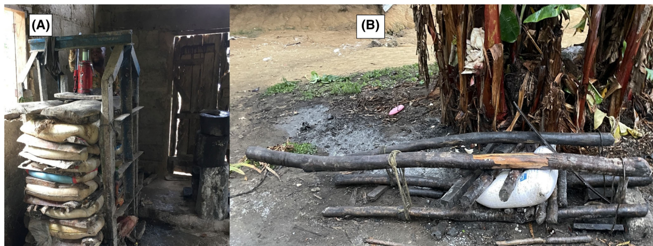
Figure 2. Grated pulp dewatering methods adopted in Nigeria (A) and Cameroon (B).
