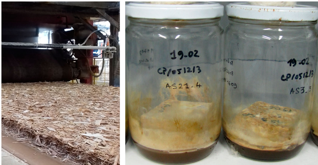
Figure 2. Left: mattress made of poplar and sweet chestnut strands entering the continuous pressing phase. Right: specimens subjected to a durability test with Coniophora puteana according to the EN113-3 standard.
