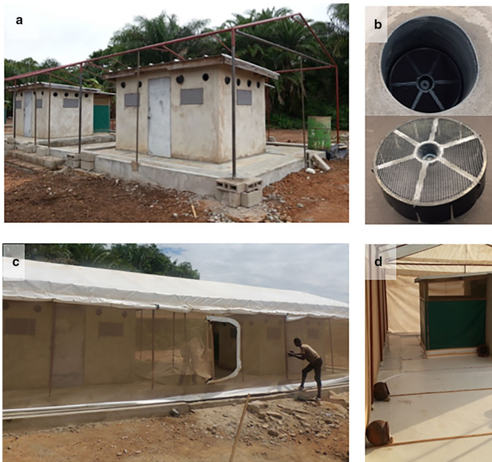
Fig. 1 Semi-field enclosure for release–recapture studies. a Metallic framework of the enclosure around 2 modified West Africa experimental huts. b Top, insert inside an EaveTube (view from outside); bottom, treated insert with visible insecticide powder. c Netting walls and door, and tarpaulin roof. d White tarpaulin floor to facilitate collection of dead mosquitoes. Six clay pots (3 visible) containing 1 l water and cotton soaked in 10% sugar solution were installed in the enclosure the morning after the release to provide resting sites and sugar sources for mosquitoes
