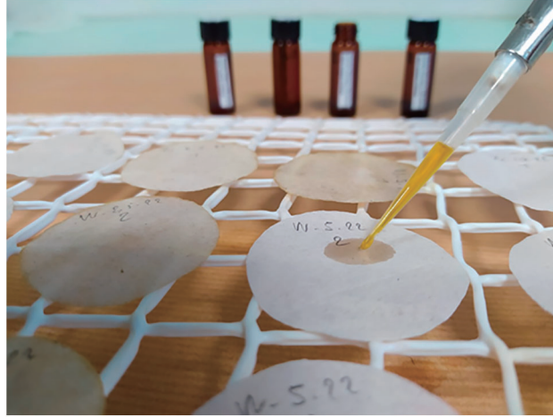
Figure 2: Impregnation of cellulosic papers prior to termite attacks
