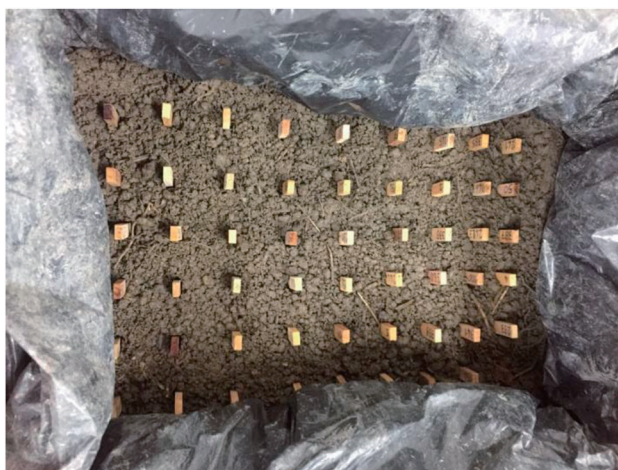
Figure 5: Laboratory test device for the unsterile soil exposures of native and impregnated Virola woods, according to the test duration
