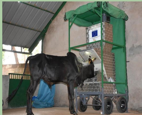
A bull calf during measurements of enteric methane emissions (GreenFeed@ device). Experimental platform of CIRDES (Burkina Faso) installed by the CaSSECS project for direct measurements of enteric methane in cattle
