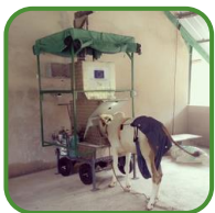
GreenFeed® – device for measuring enteric methane emissions
