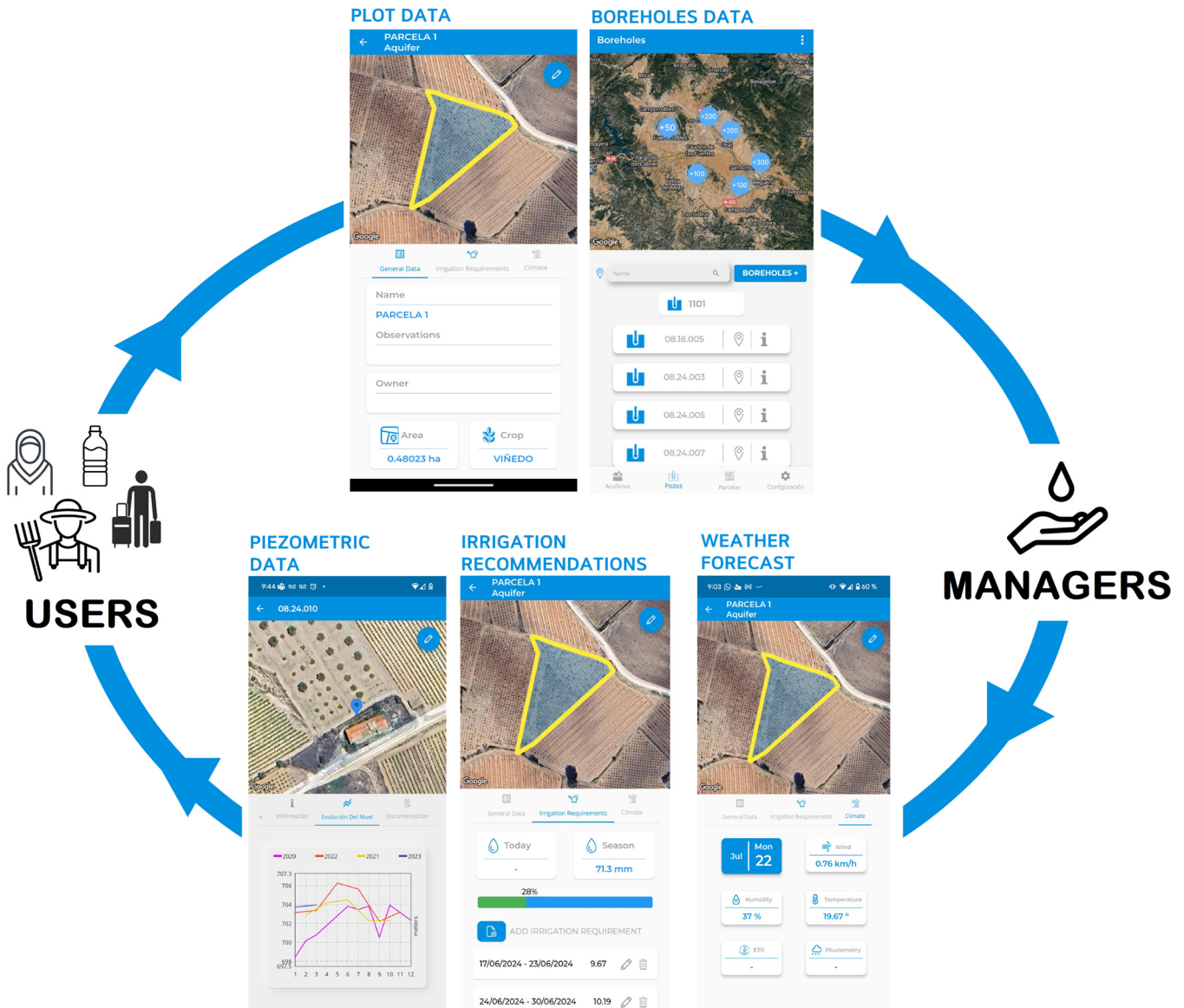
Figure 1. With the app developed (both for Android and iOS systems), users can provide boreholes and plot data to managers (above), and managers give them back hydrogeological data, irrigation recommendations, and weather forecasts (below, from left to right). All the functionalities are described at: https://www.youtube.com/watch?v=b4moFIdmF4g (accessed on 26 September 2023).
