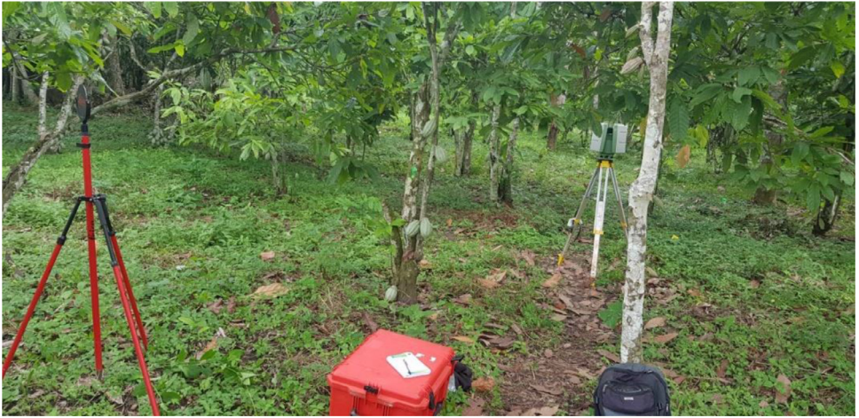
Fig. 2. Scanning a cocoa based agroforestry system in Cameroon. The scanner is in the background (in grey and green). One of the spherical targets used to adjust the successive scan positions is in the left foreground. Credit: Stéphane Momo Takoudjou.
