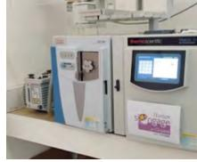
The GC-MS Trace 1610-ISQ700 coupled with the riPlus RSH Smart autosampler © R. Lehnebach, CIRAD
